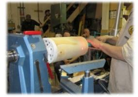
Shown here is the laser pen light just about to clear the sidewall of the vase. The laser has been set for a wall of a desired thickness with the cutter prior to inserting the cutter in the vase.
