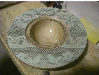
The surface above was achieved by stretching a lace table cloth tightly over the piece, and then spraying painting through the table cloth onto the piece. The paint must be thinned, and Jim uses an air brush. Spraying with spray cans does not seem to work as the paint is too thick, and too much paint (volume) is delivered by the spray can.
