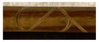
The blank above was made with three pieces of veneer laminated together, and then insert in random cuts using the same process described above.
