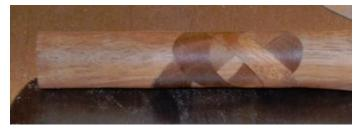
Look closely at the picture above and you will see that the sections of the knot do not line up, nor do they extend down the blank the same amount on the left hand side. This was done on purpose to show what happens when the insert is wider than the saw kerf. Remember the MOST IMPORTANT JIG!
