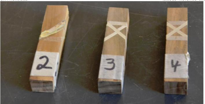
Three blanks with different number of cuts and glue-ups done in each. The blank on the far right labelled 4 is now ready to be mounted on the lathe and turned. If you were making a pen, this is the point where you would cut the blank to length, drill the blank for the pen tube, glue in the tube and then mount the blank on the lathe.
