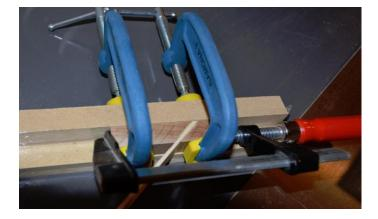
The blank and insert after the glue has set and the blank removed form the jig.
