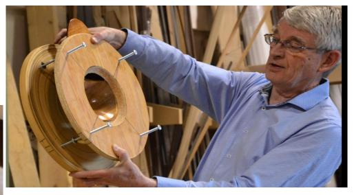
Wilf also shoed us a lidded vessel made from local hardwood. Into the vessel he inserted a segmented ring of coco-bolo so he had a good solid dense wood fur cutting threads.
