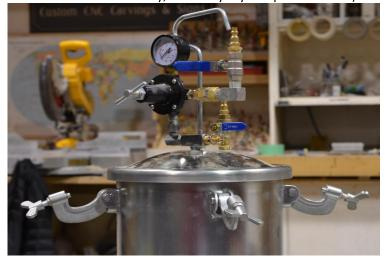
The purpose of the pressure pot is to force the resin into all of the voids in the piece.
