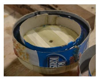
You can do the same process without using a pressure pot. To get the bubbles otu of the epoxy, use a propane torch lightly across the epoxy. The heat makes the epoxy thinner so the air can get out, and the bubbles "pop". The key is to only lightly use the torch.
