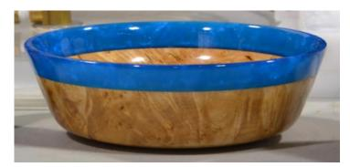
First Lyle rough shapes the bowl and makes a recess for a tenon for mounting on his chuck. Then he hot melts thin carboard to the piece to act as a mold. His mixes the epoxy, purs it into the mold and leaves it in the pressure pot for 48 hours. After 48 hours the epoxy has hardened and the piece is removed from the pressure put, finish turned, and polished. To finish Lyle sands to 400 and then applies either Mirror Coat epoxy or two to four coats of wipe on poly.
