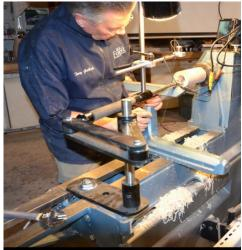
Alternate methods of using articulating arm hollowers are to have a laser shining down. The idea is that you set the gap between the laser beam and the cutter to the thickness that you want, and then cut until the laser is just on the edge of the outside of the piece. The drawback to this method is the laser does not take into account the curve of the piece, so you have to constantly adjust the laser or risk blowing through the side of the piece.
