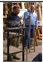
The Hopewood Turning tool is a cutter on an articulating arm. The tool that Terry demonstrated has a camera directly over the cutter, and a screen that is set up over the piece being worked on. With an overlay over the screen, terry outlined where the cutter contacts the wood. This way he could see on the screen exactly where the end of the cutter was and the remaining thickness of
