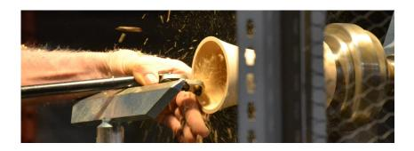
To turn the other side of the portal, Ron makes a specialized chuck to hold the turned side of the piece on the lathe so he can hollow out the other side.
