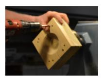
With what will become your chuck mounted on the lathe, go back to your turned piece and determine what the diameter of the turned piece is about 3/4" from the end. Hollow out the two piece block to form a collar that will fit the portal. This takes a bit of trial and error, with one piece being taken off the chuck and fitted against the portal. Once you have the pieces cut so they fit take both pieces off the chuck. These two pieces will be the outside "jaws" of the chuck.
