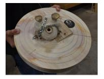
5. Put a block of wood in the chuck, and then use strings on screws to hold the piece (delicate light pieces only and very light cuts!)
