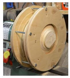
green turned and now dry (but warped) turnings, etc. Different sized donuts (disks with holes cut in them) and lengths of bolts allow you to mount different sized objects. A piece of hose or rubber tubing around the hole provides a cushion if you are worried about putting a mark on a finished surface.
