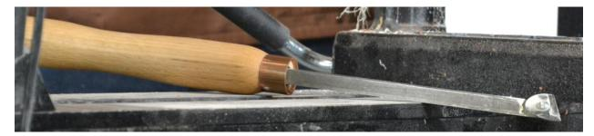
Graham then gave a demo of how to wet scrape with the tool. He had a bowl mounted to the lathe with the outside turned. He wet the outside of the bowl with a spray bottle and then lightly scraped the bowl. The shavings he got were extremely thin. He says after scraping he would let the piece dry and he gets about a 200 grit finish from the tool. He says it is a great trick to use on highly figured wood or any wood that is prone to tear out.
