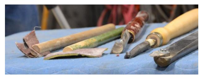
Sanding is one with a mop handle with a slot cut in it to hold the sandpaper. The urn is then parted off with a cup in the bottom so it will not rock.
