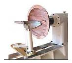
The One Way system consists of two posts that attach to the bedway of the lathe. Into one post is mounted a cutter, and into the other a cutter support. The cutter and cutter support are curved and come as a pair with the same diameter. There are four different diameter cutters available, 9", 11 ½" 13 ½" and 16 ¼".
