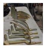
The cutters are basically a carbide negative rake scraper on a curved arm.
