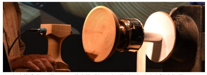
Ed made a holder for his wood burning pen. The holder slides on a board he placed on the bed of the lathe. The tip of the wood burner is shaped so that it fits around and bead. Ed orients the piece according to the indexing plate and then burns each groove horizontally. He burns the inside and then the outside of the piece. Once both the inside and outside have been burned, he rotates the piece as per his indexing wheel, and burns the next horizontal line.
